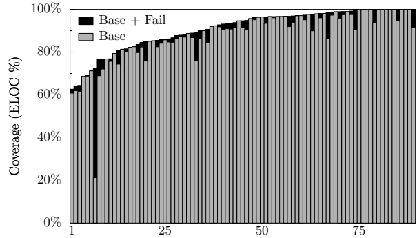
Figure 5: Line coverage for each application with and without failing system calls.
