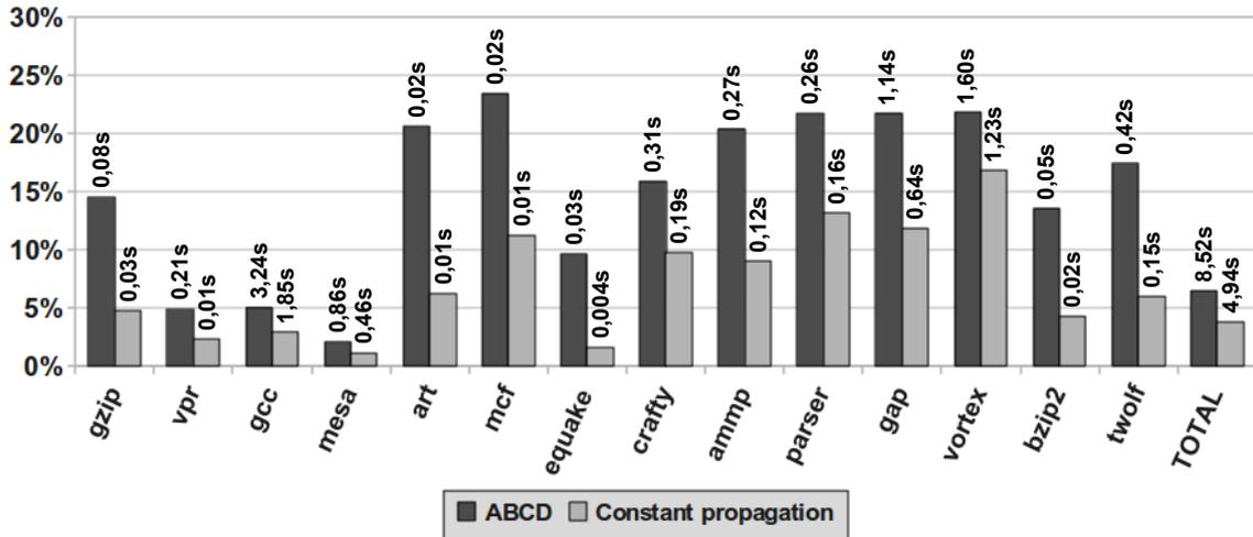
**Figure 6. Execution time of partial compared with full SSI conversion. 100% is the time of doing the full SSI transformation. The shorter the bar, the faster the partial conversion when compared to the full conversion.**
