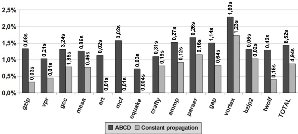
**Figure 7. Execution time of partial SSI conversion compared to the total time taken by machine independent LLVM optimization passes (`opt`). 100% is the total time taken by `opt`. The shorter the bar, the faster the partial conversion.**
