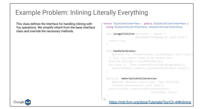
This class defines the interface for handling inlining with Toy operations. We simplify inherit from the base interface class and override the necessary methods.
