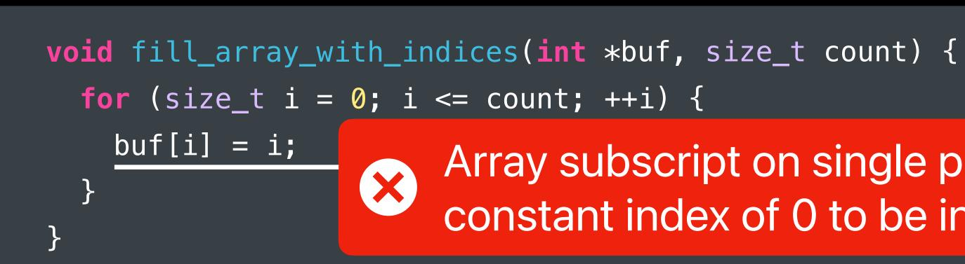
Array subscript on single pointer 'buf' must use a constant index of 0 to be in bounds
