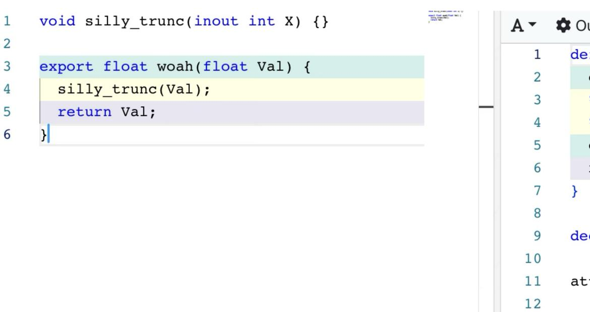
🗘 Output... 🔻 🝸 Filter... 👻 📃 Libraries 🛛 🎤 Overrides 🛛 🕂 Add new... 👻 🥒 Add tool... 💌 define float @"\01?woah@@YAMM@Z"(float %Val) #0 { call void @llvm.dbg.value(metadata float %Val, i64 0, metadata ! %1 = fptosi float %Val to i32, !dbg !32 %2 = sitofp i32 %1 to float, !dbg !32 call void @llvm.dbg.value(metadata float %2, i64 0, metadata !29 ret float %2, !dbg !33
