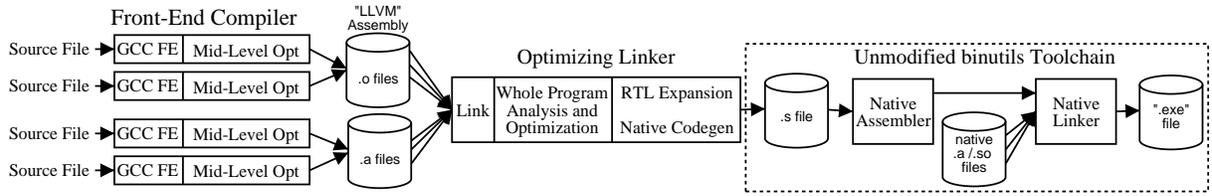
Figure 1: High-Level Compiler Architecture for Whole-Program Optimization
