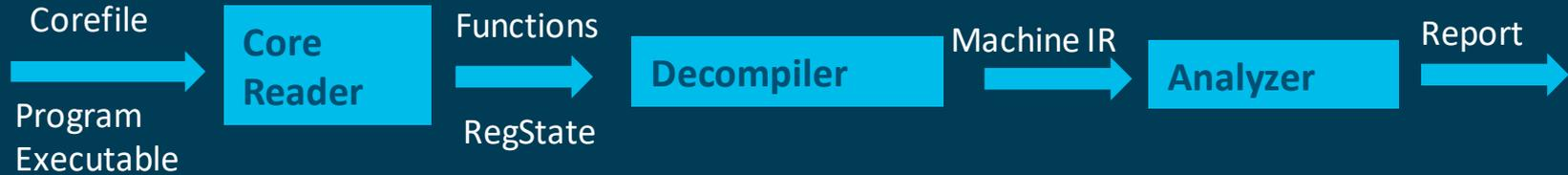
**Core Reader** - extracts functions, registers, memory state from the backtrace of the crashing thread.
